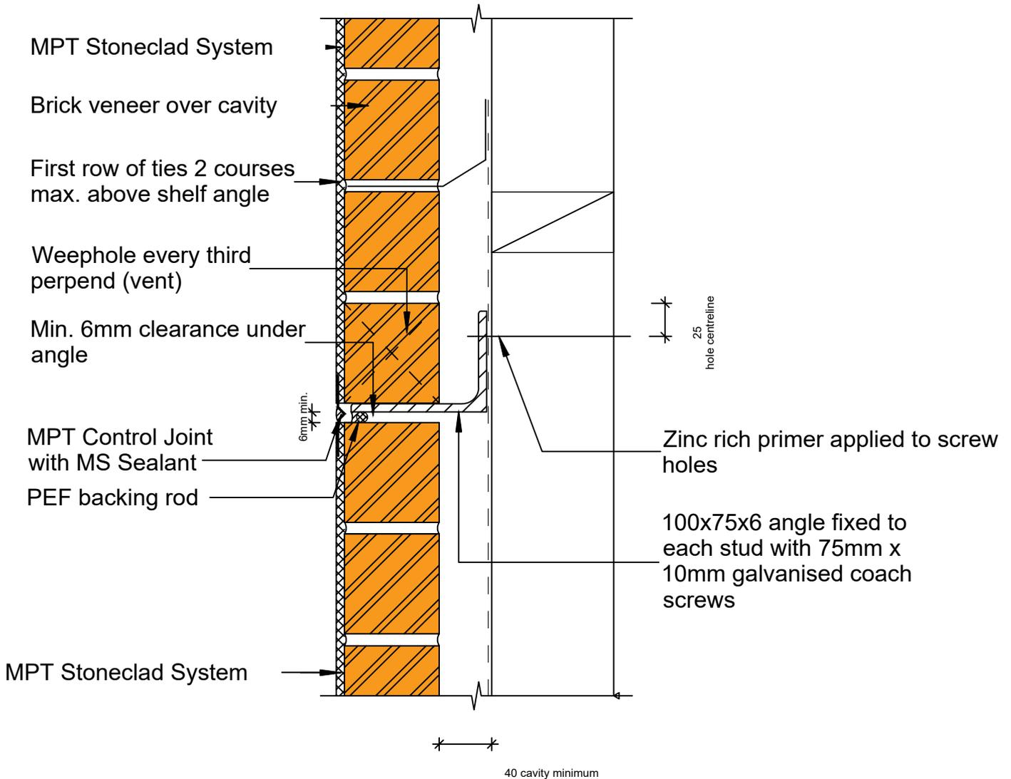
Note that the Brick Two Storey Solution covered in Design Note C1 does not require the use of shelf angles if slip joints are used, however they may still be a preferred option in some circumstances
